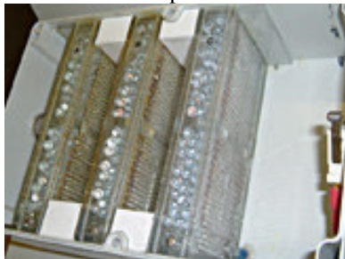
Figure 3: Non-Thermal Plasma Oxidation Unit
